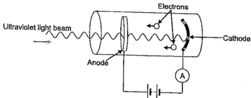
The largest wavelengths of monochromatic light that will cause the ejection of photoelectrons in the above photocell is 229 nm. When a person interrupts the beam, the sudden drop in current activates a switch, which sets off the alarm.
