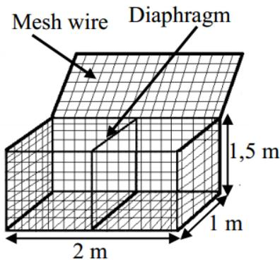
Farmers decide to build a bigger gabion basket but to keep the ratio of the dimensions of the original gabion basket the same, that is L : B : H = 2 : 1 : 1,5. Calculate the volume of the bigger basket if the new breadth is 1,75m
