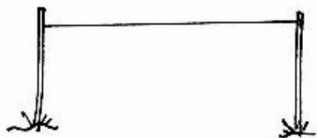
The line is made of wire, that won't stretch. When there is no washing on the wire, the wire is almost straight. But now look at this diagram [below]. . . when a wet towel that weighs 20 N is hung in the middle of the line,
